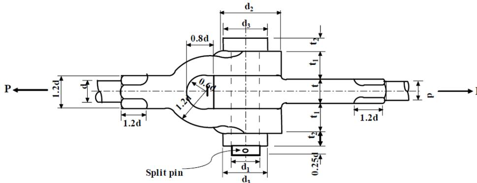
Fig. 1 A typical knuckle joint
